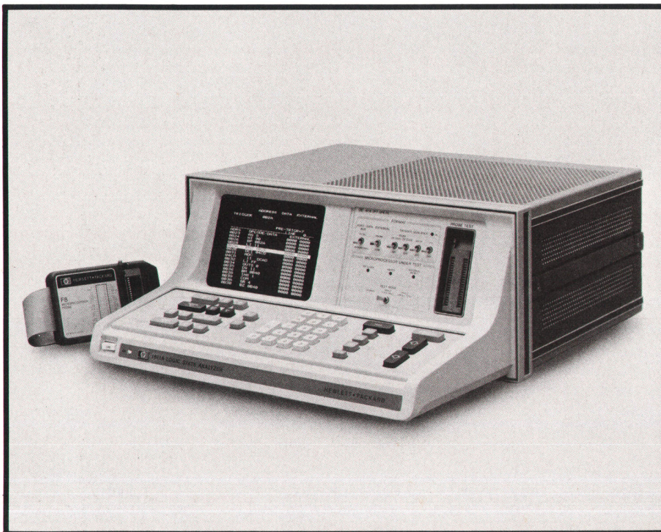
Fig. 1. Model 1611A Logic State Analyzer uses "personality" modules to configure the instrument for testing digital systems designed around particular microprocessors. Each personality module establishes the appropriate pin connections for the probe, sets the proper clock slope and threshold levels, and encodes the microprocessor's data bus contents into the mnemonic code used for that microprocessor.
