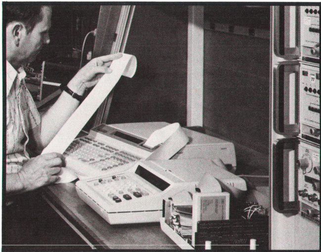
Fig. 5. Model 1602A, shown here with a Model 9825A Desktop Computer, is programmable by way of the HP Interface Bus and is thus easily adapted to automatic test systems.
